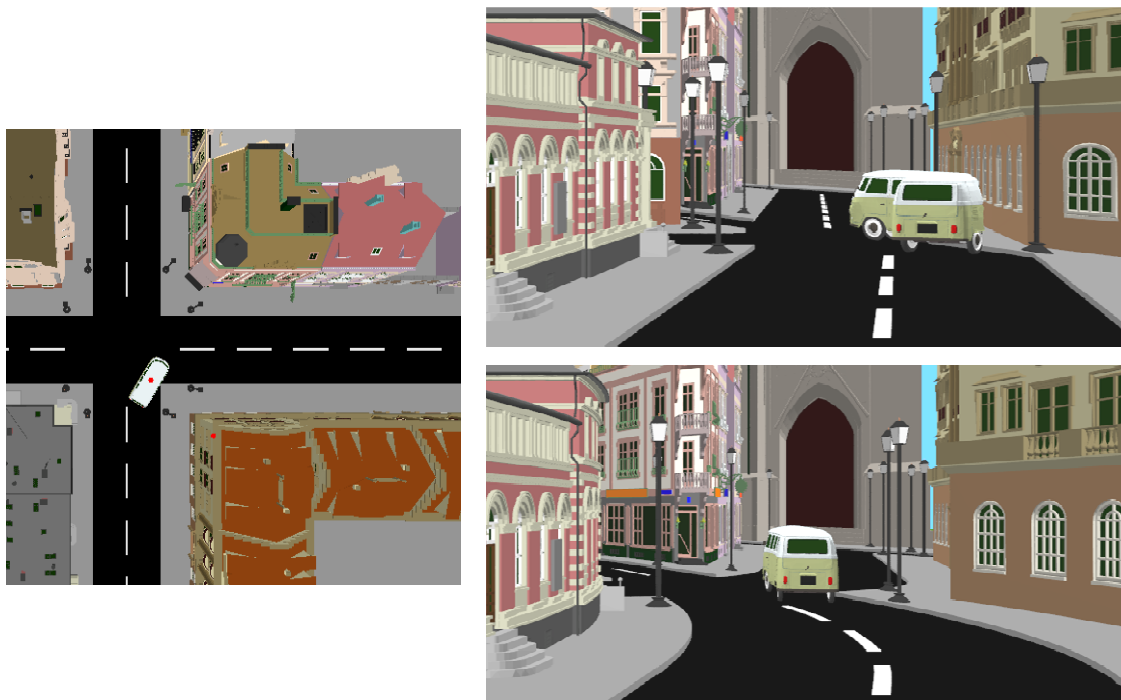
Figure 1.10. Graph camera continuity illustration. The graph camera ( top ) produces has an abrupt change of perspective while the curved ray camera ( bottom ) minimizes the local distortion such that it is almost not visible.
