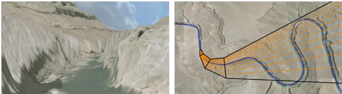
Figure 1.11. A curved ray camera used to linearize a path. A curved ray camera ( left ) allows forward and backward navigation along a user defined path ( right ).
