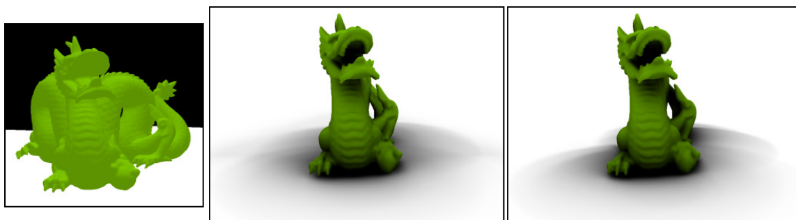
Figure 4.3. An ambient occlusion example. A graph camera depth buffer illustrated with color ( left ) is used to render the ambient occlusion effect ( middle ) and compared to using a PPC depth buffer ( right ). The graph camera captures hidden parts of the dragon for a more complete and stable shadow.
