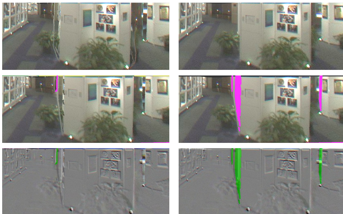
Figure 1.9. Occlusion camera application to image compression. Top : Occlusion camera image ( left ) used to compress a single image ( right ) from the sea of images. The occlusion camera image and a planar pinhole camera image ( not shown ) are warped to the output viewpoint location ( middle ) and a residual is calculated ( bottom ).
