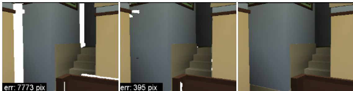
Figure 3.15. A depth discontinuity occlusion camera example of the Unity. A three-way comparison between reconstructions that use a PPC reference image ( left ), DDOC reference image ( middle ), and the original scene geometry ( right ).
