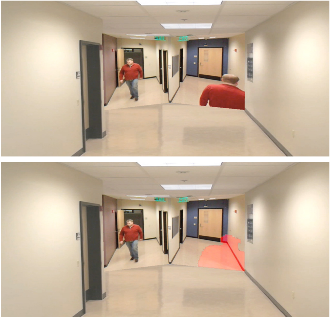
Figure 4.26. Illustration of near clip plane by background subtraction. The back of the subject is sampled by the camera that is supposed to sample the right branch of the corridor ( top ). The back of the subject is erased using a background image of the corridor acquired before the subject appeared ( bottom ).
