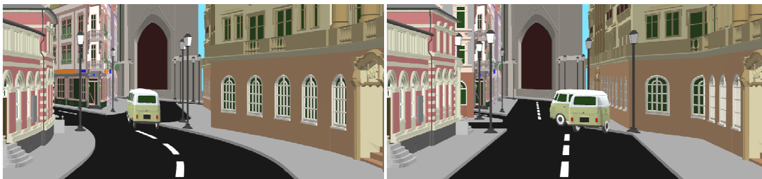
Figure 4.8. Distortion comparison between the curved ray camera and graph camera. The CRC visualization ( left ) minimizes the distortion through the perspective transition region as opposed to the graph camera which switches abruptly between viewpoints ( right ).
