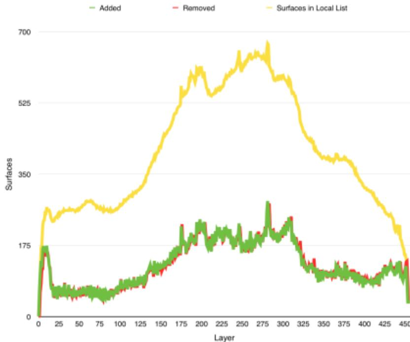
Fig. 4: Surface patch utilization of the local list: the number of added and removed surfaces are shown in green and red, respectively, while the total active surfaces are marked in yellow.
