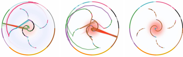
Fig. 8. The material point method (MPM), a particle-based mechanical engineering simulation, in action. Left: Computation of momentum from the mass and velocity data (in the black and green arrays). The algorithm tends to sweep through the values in order, resulting in good cache performance. Middle: Computation of the particle stress update (brown data array) near the end of the timestep, from various data, including the constitutive model (blue data array). MPM is made up of several phases which tend to access the data in order. The resulting visual pattern is that of data moving into L1, being operated upon a limited number of times, and then slowly migrating first to L2 and then back into main memory, as newer data comes into L1 to be operated upon in turn. Right: This example uses a larger example with a larger cache to demonstrate the scalability of our visualization system.
